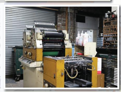
An offset press; a quick and efficient machine for printing book interiors
